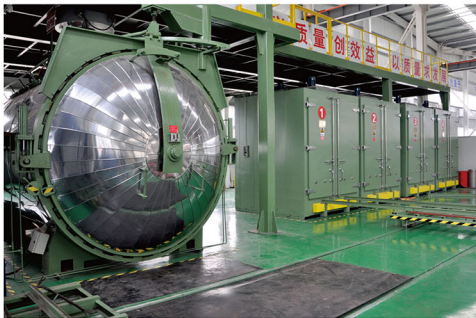
真空浇注设备及固化炉 Vacuum casting equipment and curing furnace
